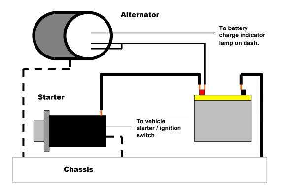
The chassis acts as an earth and provides a return path for the electricity to the battery negative terminal.
