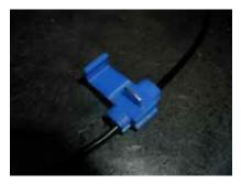
Slip the connector over the alternator wire (Black in this case).
