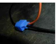
Use a pair of pliers to depress the metal spade into the body of the connector. This metal spade has blades which cut through the insulation of the wire making contact with the inner conductor.
