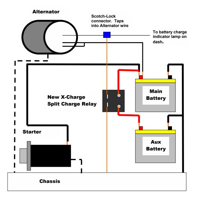
New wire colours are shown as supplied in the X-Charge kit.
