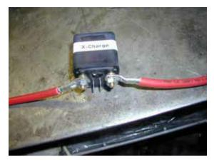
The heavy red leads are used to connect the two stud terminals on the X-Charge Relay to the batteries. The leads are supplied with a ring connector on each end. The smaller ring attaches to the split charge relay.
